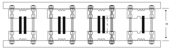
H = L + 64mm (for 10p, 11p, 12p, 14p Series) H = L + 44mm (for 20p, 21p, 22p, 24p Series)
